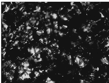
图 4 偏光显微镜观察的玻纤分布情况 Figure 4 Glass fiber distribution inside the polymer matrix observed by POM
